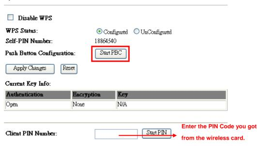
(3.) Back to "Wireless Utility" and press the "Start PIN" button to complete the auto-paring process.
