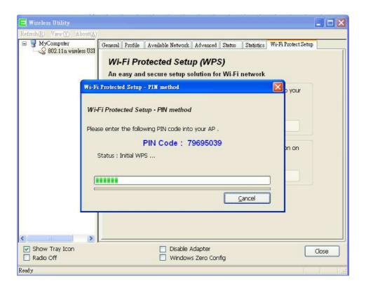
(2.) Open menu "Wi-Fi Protected Setup" of RB-1732 Broadband Router, input the PIN number from the wireless card then click **Start PIN**.
