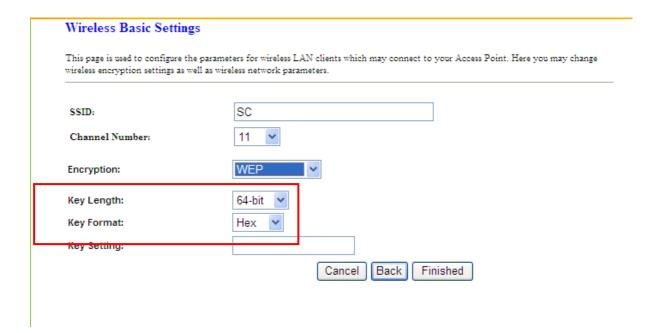
**Key Length:** For 64bits WEP key, 10 hexadecimal digitals leading by **0x** can be entered. For 128bits WEP key, 26 hexadecimal digits leading by **0x** can be entered.
