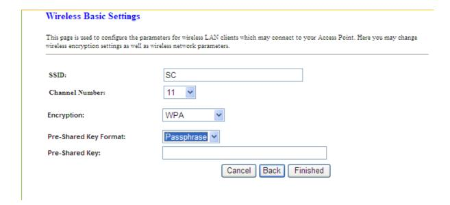
WPA (TKIP) and WPA2 (TKIP): Allow the access from WPA clients simultaneously and the encryption keys are given from PSK respectively.
