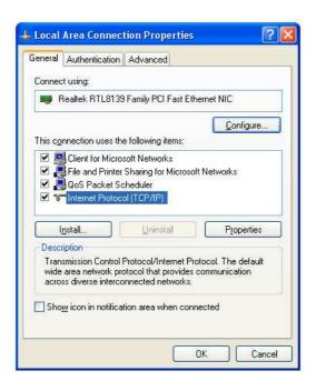
**Step 4-1.** For getting IP automatically if you are one of the users under RB-1732 Broadband Router, please skip **Use the following IP address** and then select **Obtain an IP address automatically** and **Obtain DNS server address automatically** and then click on **OK** button.
