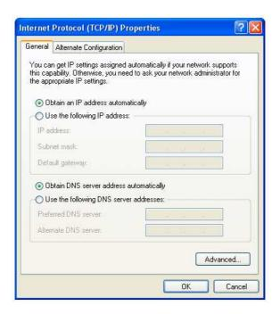
**Step 4-2.** For getting IP manually in order to specify a Virtual Server, such as Print Server, FTP Server and so on, please skip **Obtain an IP address automatically** and then select **Use the following IP address**. And the following default setting of RB-1732 Broadband Router should be noted:
