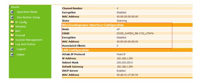
**Step 2.** Setting the same SSID, channel and security you got form "Network Config" and Click on **Apply Changes** to save the setting
