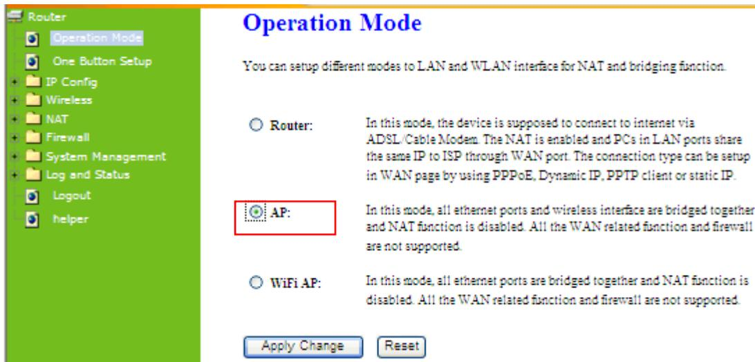
When this product is used as an access point, the IP address has to be changed. The default IP under AP mode is 192.168.1.254.
