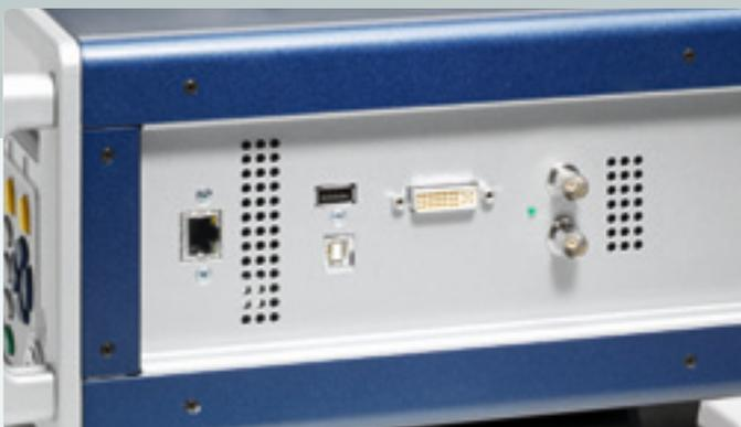
**All interface in review:** Ethernet RJ45, ASI in/out over BNC, USB-A, USB-B, SCART, DVI out.
