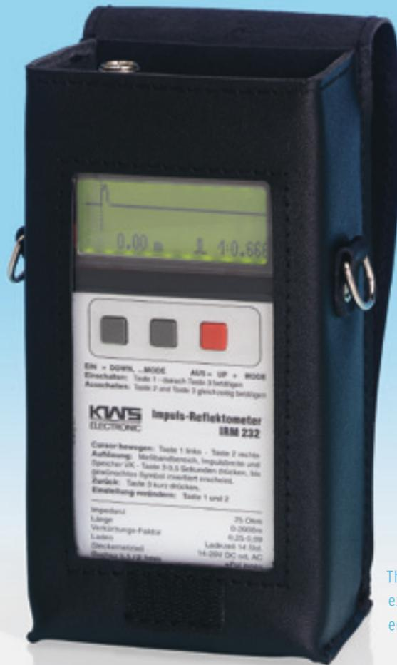
The Pulse Reflection Meter IRM 232 locates irregularities, exposed lines and short circuits in antenna, data and energy lines.
