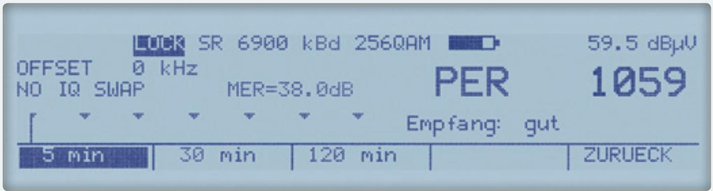
The principle of success, to use 2 separate displays is also in the AMA 310. The new LC-display for measurement display is bright and can also be read in very light surroundings.
